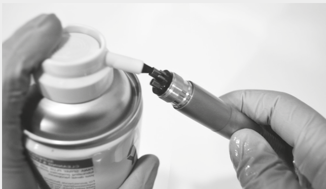
Injecting maintenance oil into the spray channel (maintenance oil item no. 174010 and spray channel adapter item. no. 17401150)
