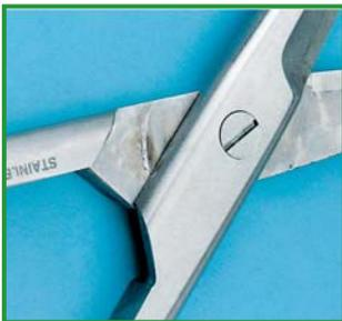
Fretting corrosion due to inadequate lubrication
