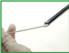
Cleaning the lens of an endoscope
