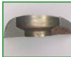
Breakage at countersunk screwhead
