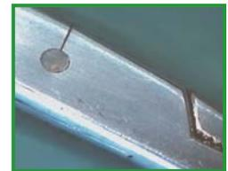
Fracture at hinge pin
