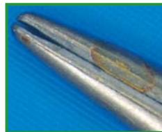
Acid attack on welds and hard metal inserts, with consequential damage in the form of extensive wear
