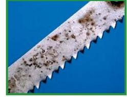
Rust formation on a chromium-plated saw blade made of carbon steel.
