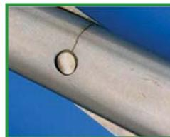
Fracture at hinge
