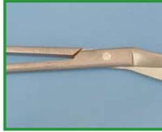
Stainless steel instrument with acid attack (brown tarnishing).
