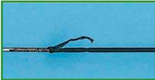
Damaged insulation on HF instrument
